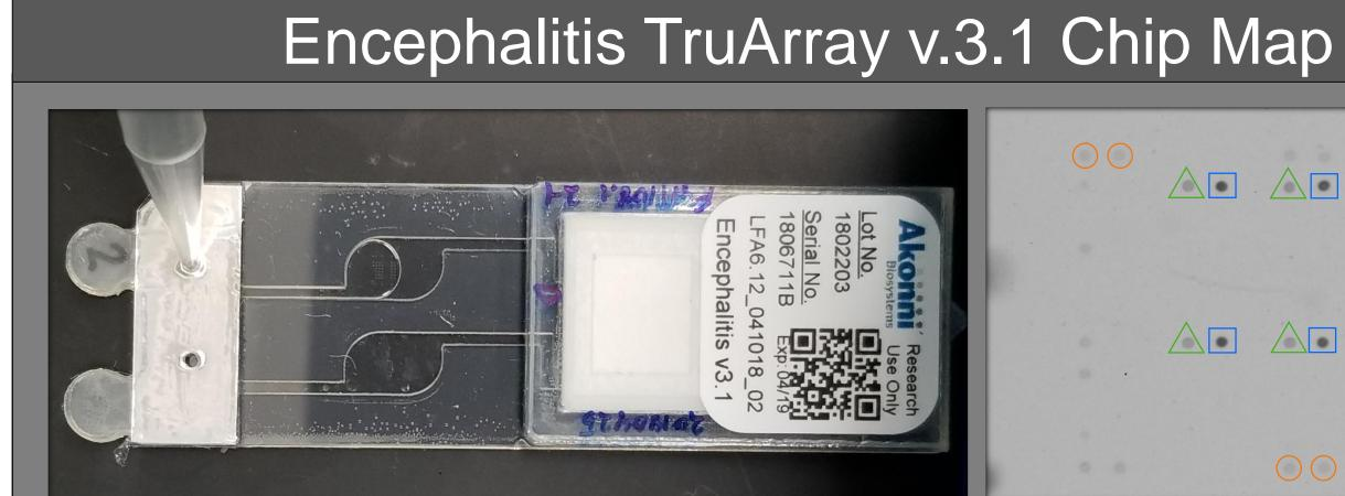
(Left) Sample loading and LFA washing conducted through a single port onboard the array
