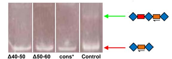
Figure 7. Negative priming assay results for all three CRISPR I leader sequence mutants. Wild type CNC was used as a control. Red Arrow = unexpanded array Green Arrow = expanded array
